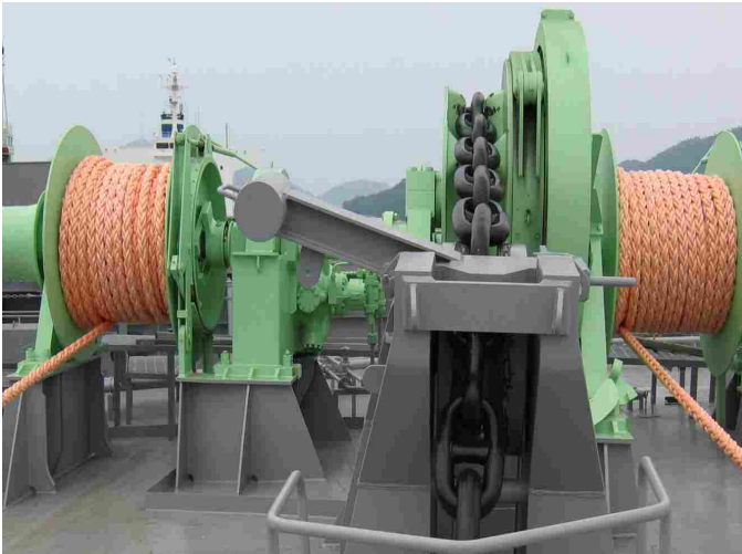
76000T 散货船用的Φ76液压锚机 Φ76 Hydraulic Windlass for 76000T Bulk Carrier
