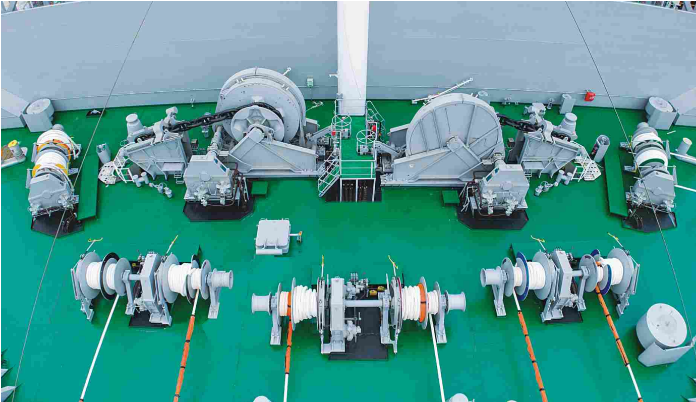
24000TEU船用Φ147液压锚机 Φ147 Hydraulic Windlass for 24000T Vessel
