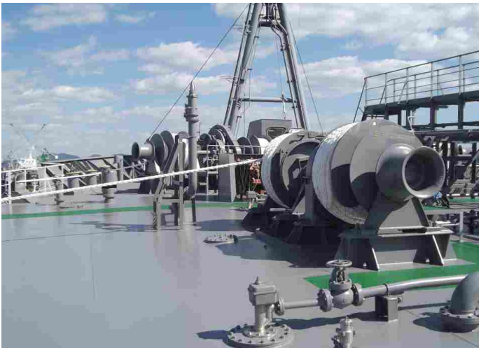
50000T 成品油船118KN 液压系统泊车 118KN Hydraulic Mooring Winch for 50000T Products Tanker
