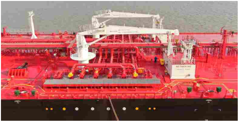
15T19M液压软管吊机 15T 19M Hydraulic Hose Handling
