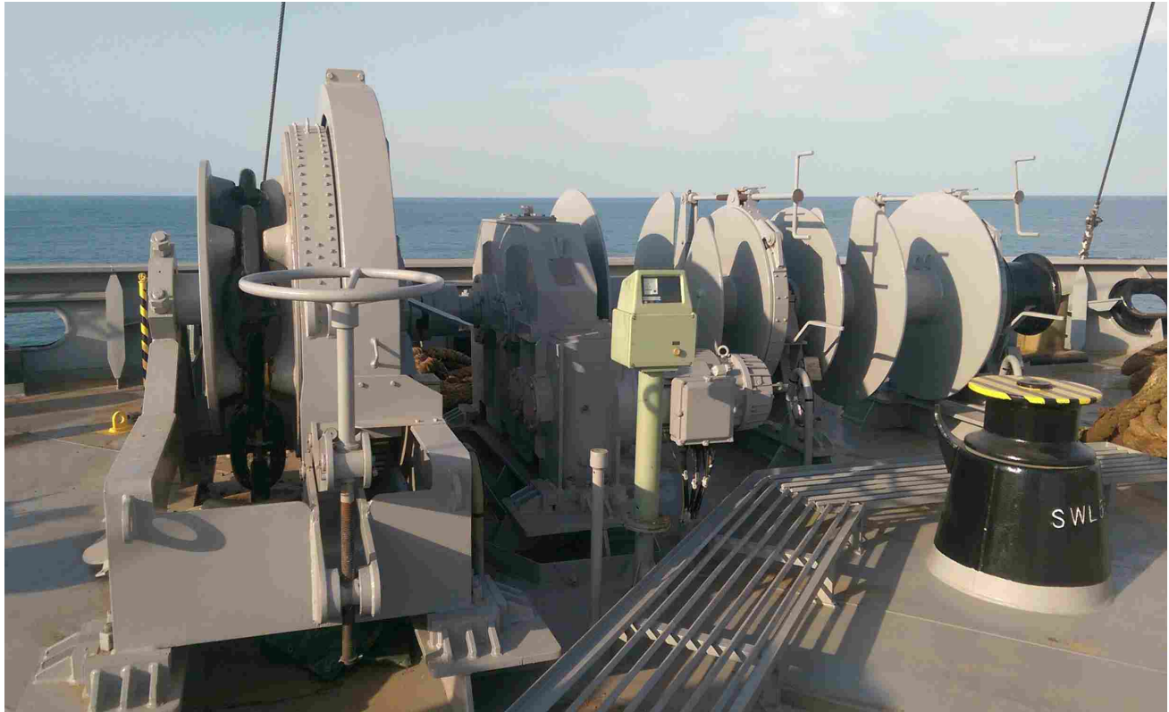
38800DWT散货船用Φ68电动锚机 Φ68 Electric Windlass for 38800DWT Bulk Carrier
