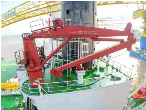
瓯洋海工风电安装船用折臂吊 Hydraulic knuckle telescopic boom crane for Ouyang offshore
