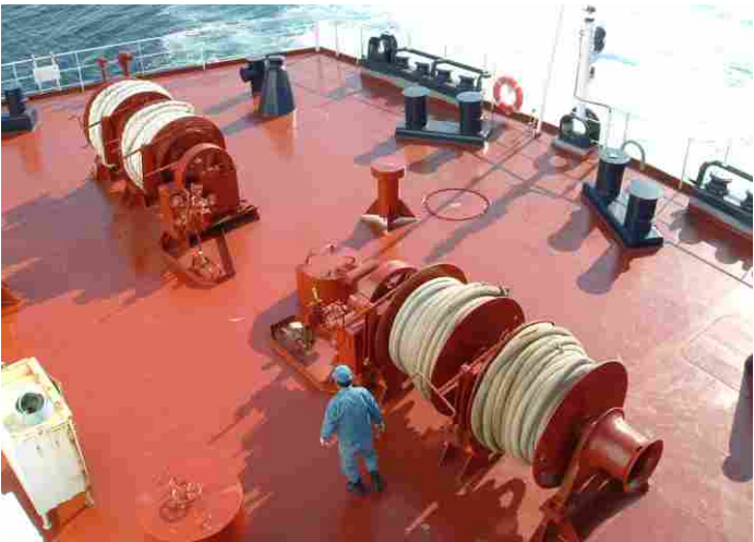
76000T 散货船147KN 液压系统泊车 147KN Hydraulic Mooring Winch for 76000T Bulk Carrier
