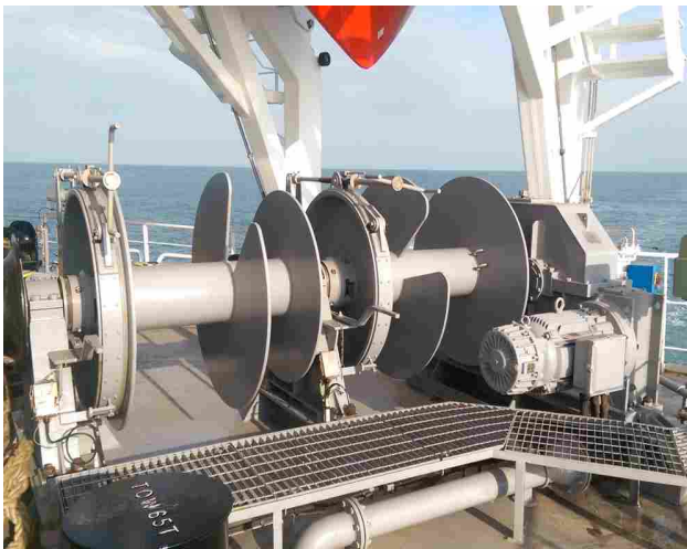
38800DWT散货船用125KN电动绞车 125KN Electric Winch for 38800DWT Bulk Carrier
