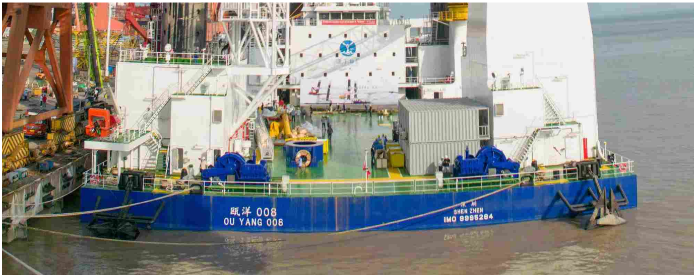
新一代深远海自升式风电安装运维平台——OY-SEU800 锚泊定位系统 A New Generation of Deep Offshore Jack-up Wind Power Installation, Operation and Maintenance Platform--OY-SEU800 Anchor Positioning System
