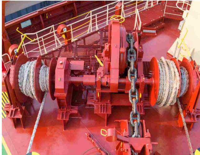
40000T油轮用Φ73液压锚机 Φ73 Hydraulic windlass for 40000T oil tanker
